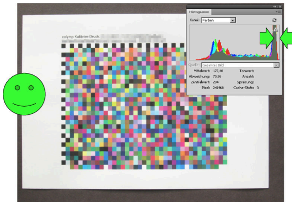
Figure 7: This is how the photograph of the test chart should be: paper is neutral white, no shadows, exposure is just right (in the histogram, the peak of the paper is slightly away from the right edge, see arrows)
