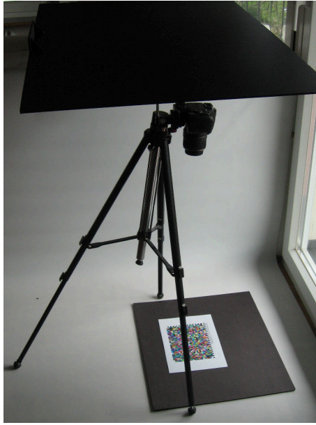
Figure 47: Avoiding reflections: black cardboard behind the camera
