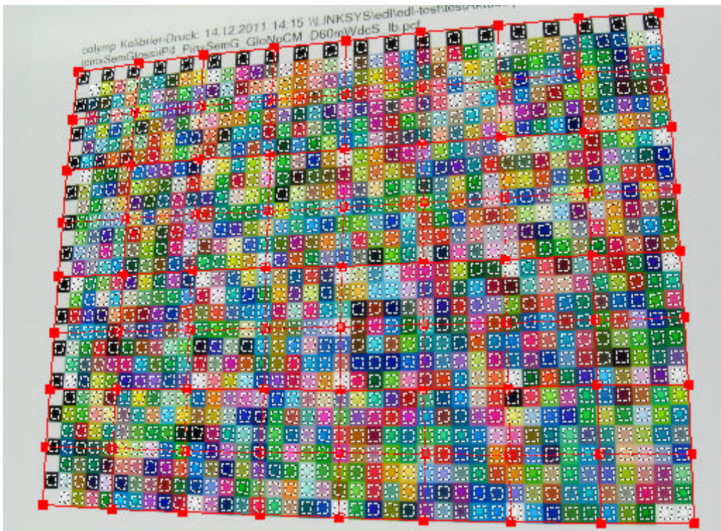
Figure 13: With colymp you can also evaluate strongly distorted photographs (in the background the photograph, in the foreground the template): The white dashed evaluation fields each lie exactly within the associated color field.
