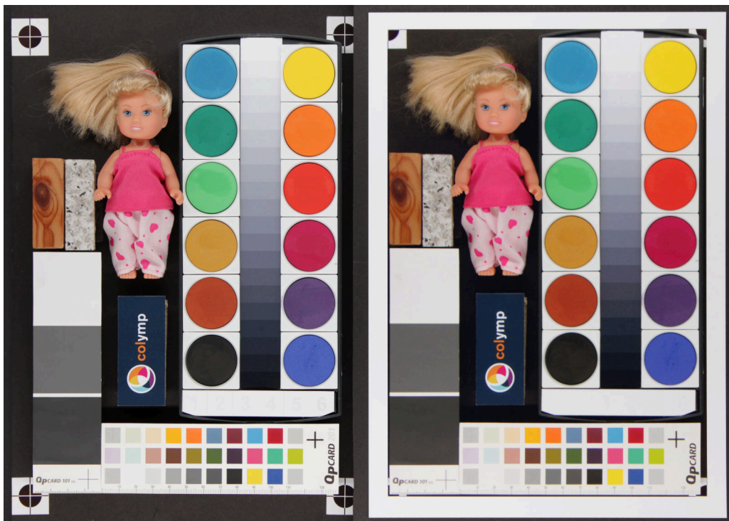
Figure 49: Example of faithful reproduction using colymp . On the left the original, on the right the printout. The printout seems to be slightly darker at the right edge, because the artificial light used for the overall image was slightly less intense on the right.
