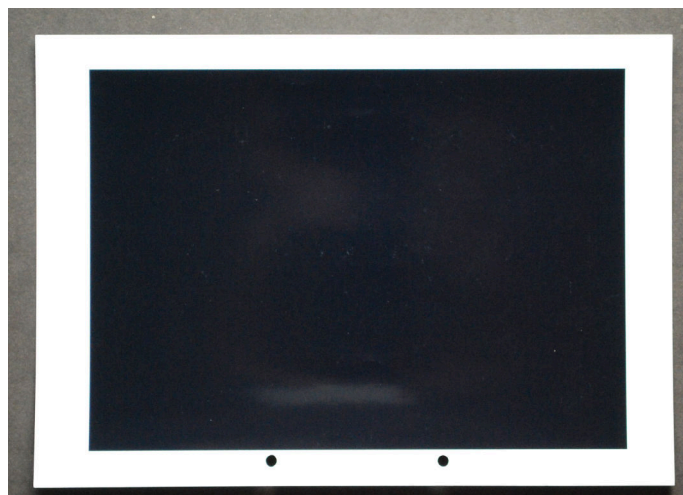
Figure 45: Disturbing reflections on black printed glossy paper (photo is overexposed to enhance the effect)
