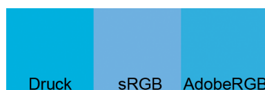
Figure 31: Example to the limitations of sRGB: Printed cyan hue, (best possible) representation of this color value in sRGB as well as in AdobeRGB. You can see that the hue in sRGB is considerably less saturated as well as brighter. (Note: all color values in this illustration are artificially desaturated and lightened to allow display on common monitors. However, the color differences roughly correspond to reality.)
